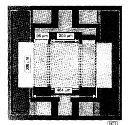
Fig. 3 Photograph of two-gap tunable MEM capacitor with firm anchoring
