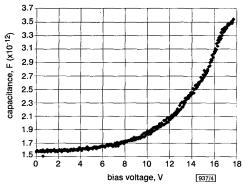
Fig. 4 Measured capacitance against voltage behaviour of two-gap MEM capacitor
