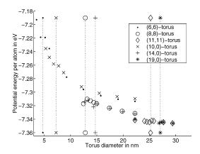
Fig. 3. Critical buckling diameter of (6,6)-, (8,8)-, (11,11)-, (10,0)-, (14,0)-, and (19,0)-tori. The buckling radius is marked by a vertical dotted line marked by the symbol representing the tube.
