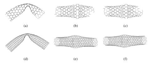
Fig. 4. Sample bends in buckled nanotori of a (10,0)-torus with 1560 atoms ((a)-(c), side, inside and outside views, respectively) and similarly an (8,8)-torus with 4608 atoms ((d)-(f)). The hexagonal bonding configuration is deformed but otherwise intact. The images of the (10,0)-and the (8,8)-tube sections are not in the same scale because of different diameters.
