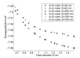
Fig. 1. Potential energy curve of relaxed toroidal structures as function of tube diameter for different torus diameters D. At about 1.35 nm tube diameter there appears a small kink for tori 22 nm in diameter.
