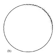
Fig. 6. Two (8, 8)-tori with different diameters simulated for 3000 fs at different temperatures. (a) D = 22 nm, T = 1500 K; (b) D = 220 nm, T = 5500 K. In (a) bond breakages can be seen but the structure remains toroidal. If the temperature is raised more, the toroidal structure breaks apart. In (b) bond breakages have evolved further and a part of the torus has already dissolved.
