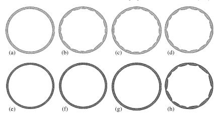
Fig. 2. Minimum energy configurations of nanotori 22 nm in diameter for different tube diameters d. (a) (17,0)-tube, d=1.33517 nm; (b) (18,0), 1.41328 nm; (c) (19,0), 1.49130 nm; (d) (20,0), 1.56938 nm; (e) (8,8), 1.08789 nm; (f) (9,9), 1.22300 nm; (g) (10,10), 1.35828 nm; (h) (11,11), 1.49344 nm. When the tube diameter d increases a structural change is observed. The onset of buckling appears as a small kink in the potential energy curve of Fig. 1.
