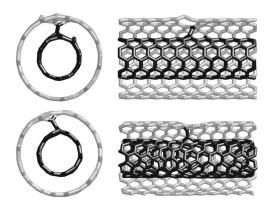
FIG. 2. Two views of a covalent intershell bond in tubes with different chiralities. Such bonds can be formed, for example, due to on-shell vacancies or intershell interstitials. The bonds shown are due to vacancy-pair reconstructions. As can be observed, the bond orientation is chirality dependent and there are several possible orientations in each particular tube.
