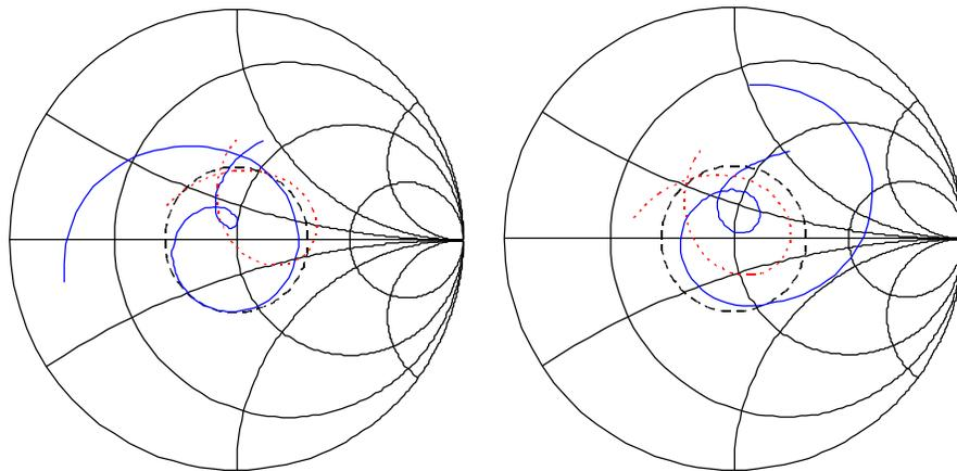
Fig. 4. Input impedance of port 1 (on the left) and port 2 (on the right). — measured,  $f = 9.5\text{--}13.5$  GHz, ..... simulated,  $f = 10.20\text{--}13.25$  GHz. Dashed circle indicates VSWR = 2.
