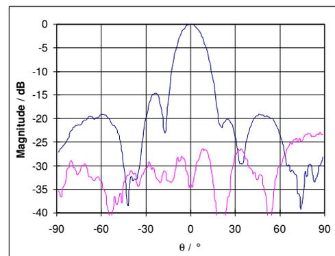
Fig. 7. Copolar and crosspolar H-plane radiation pattern of the  $4 \times 1$  - array. Port 2.  $f = 11.725$  GHz.
