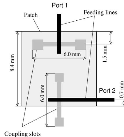
Fig. 2. Geometry of the antenna.
