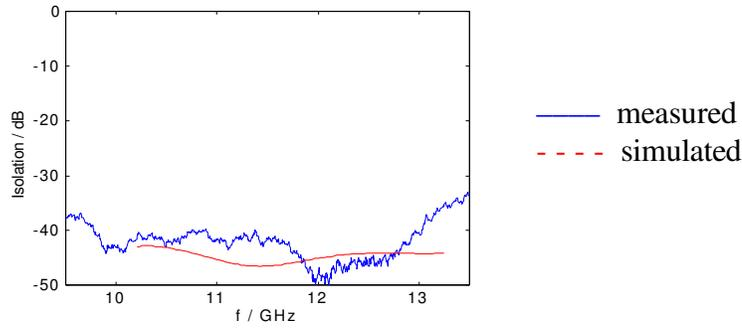
Fig. 3. Isolation between ports 1 and 2.
