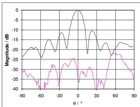
Fig. 6. Copolar and crosspolar E-plane radiation pattern of the  $4 \times 1$  - array. Port 1.  $f = 11.725$  GHz.
