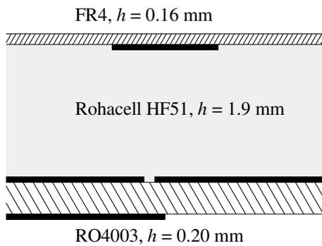
Fig.1. Layers of the antenna.
