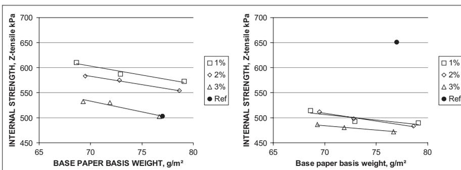
**5. Z-tensile internal strength for base paper (left) and surface-sized paper (right).**
