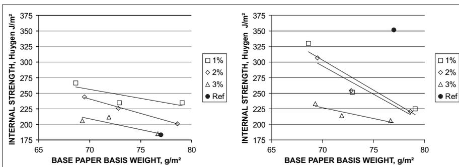
**4. Huygen internal strength for base paper (left) and surface-sized paper (right).**
