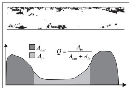
**1. Derivation of the starch penetration curves and dimensionless penetration number from 16 cross sections stained with iodine and normalized for thickness.**
