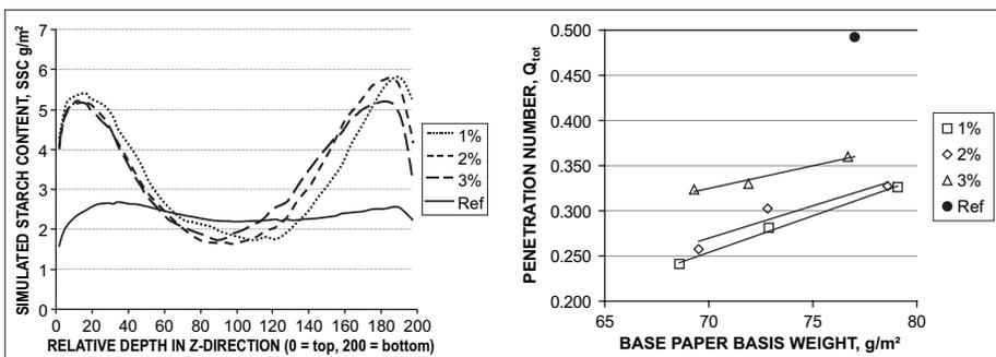
**2. Starch penetration for the reference and trial samples as characterized by SSC distribution (left) and penetration number  $Q_{tot}$  (right).**
