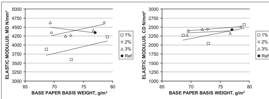
**7. Elastic modulus of the base sheet in the machine (left) and cross-machine directions (right).**
