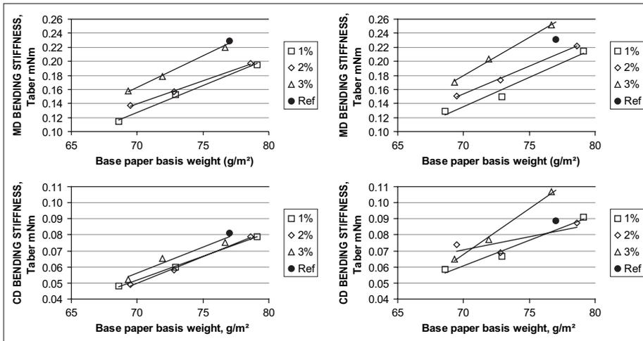
**6. Taber bending stiffness for base paper (left) and surface-sized paper in the machine direction (top) and cross-machine direction (bottom).**
