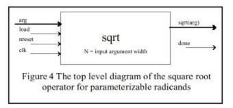
The modified Dijkstra's square root operator for 16- bit unsigned integers was compiled for Altera's 10K50 target device [7]. The device utilization and performance of the modified Dijkstra's square root operator is presented in Table 1 .The latency of the modified Dijkstra's square root operator is only 8 clock cycles for 16-bit radicands.
