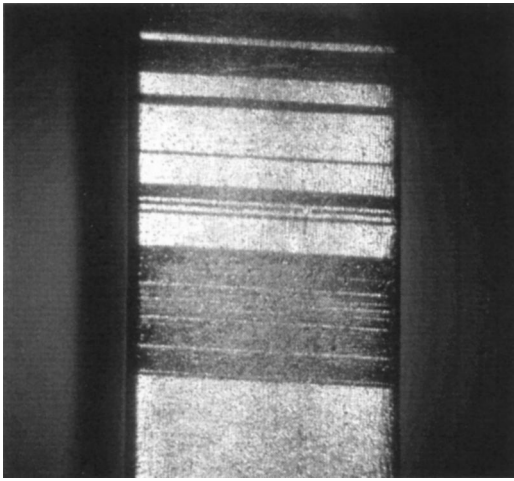
FIG. 5. Optical micrograph of the twin boundary structure of the studied MSM material at 1.8% strain. The two variants can be seen as dark and light areas on the surface.
