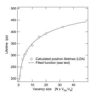
FIG. 9: The calculated positron lifetime as a function of the number of vacancy pairs. The solid line is a fit of a function, where the electron density n is inversely related to the vacancy cluster size.
