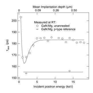
FIG. 5: The average lifetime of positrons as a function of incident positron energy in the unannealed GaN:Mg sample. The p-type Ga:Mg sample is used as a vacancy free reference. The solid line is to guide the eye.
