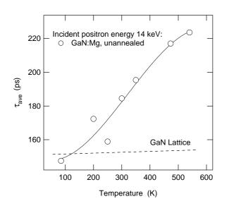
FIG. 6: The average positron lifetime of unannealed GaN:Mg sample as a function of measuring temperature. The incident positron energy was 14 keV. The solid line is to guide the eye.
