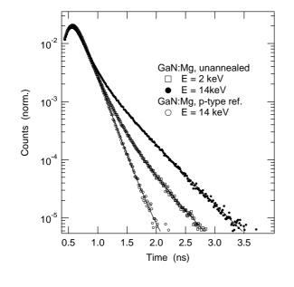
FIG. 8: Positron lifetime spectra in the unannealed GaN:Mg sample measured with two different positron energies at 540 K. The Mg-doped MBE grown p-type sample is shown as a vacancy free reference. The area of each spectrum was scaled to 1. Solid lines are the fitting results of respective spectra.
