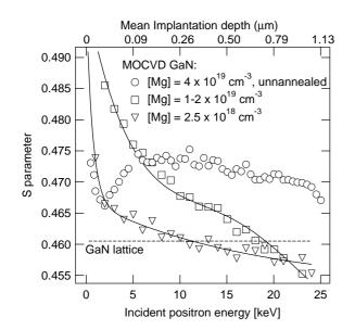
FIG. 2: The valence annihilation parameter S as a function of incident positron energy in GaN layers. The samples were annealed at 800  $^{\circ}$ C except the one with highest Mg concentration. The dashed line represents the S parameter level of annihilations of delocalized positrons in the GaN lattice. The top axis indicates the mean implantation depth of incident positron. The solid lines are to guide the eye.
