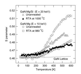
FIG. 4: Valence annihilation parameter S as a function of measuring temperature. The incident positron energy was chosen high enough to make sure the annihilations arising from the surface are excluded.
