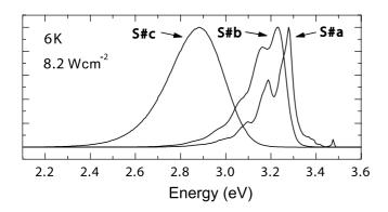
FIG. 1: Normalized low temperature PL spectra of three GaN:Mg epitaxial films deposited by MOCVD on a-face sapphire substrates. Note the line shape change and the red-shift of the peak position with increasing Mg concentration, from  $2.5 \times 10^{18}$  to  $7 \times 10^{19}$  cm<sup>-3</sup>. These samples have been postgrowth thermal anneal at 950 °C. The spectra are corrected for instrumental response.
