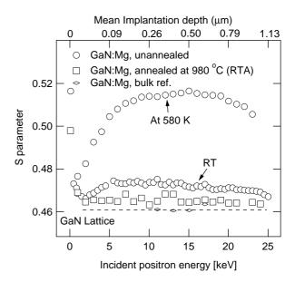
FIG. 3: The valence annihilation parameter S as a function of incident positron energy in annealed and unannealed GaN:Mg sample with Mg concentration of 4  $\times$  10<sup>-19</sup> cm<sup>-3</sup>. The p-type GaN:Mg is used as vacancy free reference. The top axis indicates the mean penetration depth.
