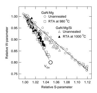
FIG. 7: The core annihilation parameter W as a function of valence annihilation parameter S measured at different temperatures.  $V_{Ga}$  represents positron annihilation parameters at Ga vacancy. Note, that the data are the same as in Fig. 4.
