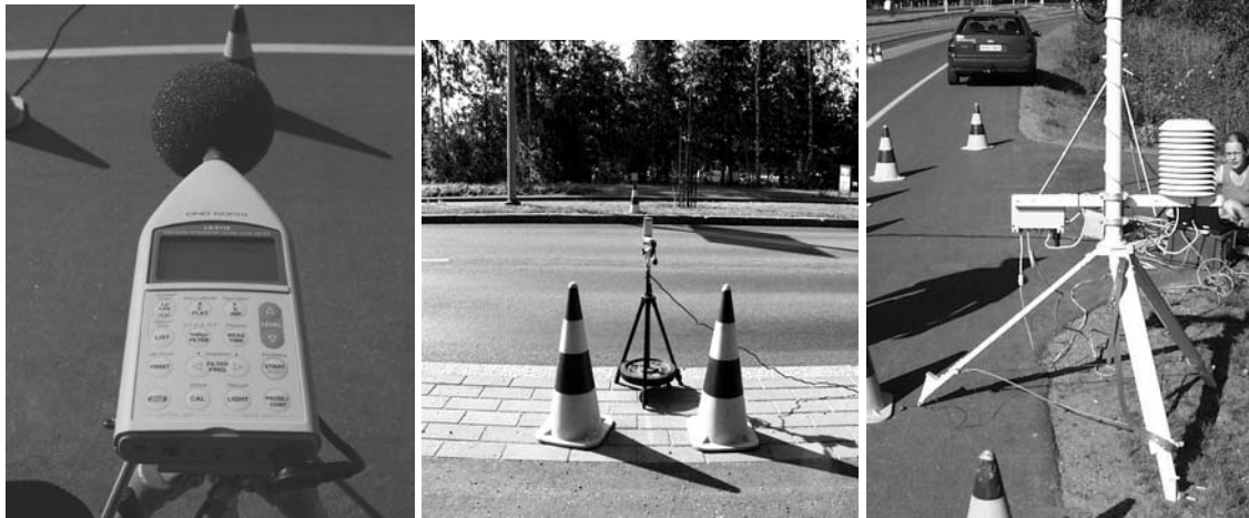
Figure 17: SPB mod -devices used: Onosokki-sound level meter, one of two laser ports and Vaisala weather station
