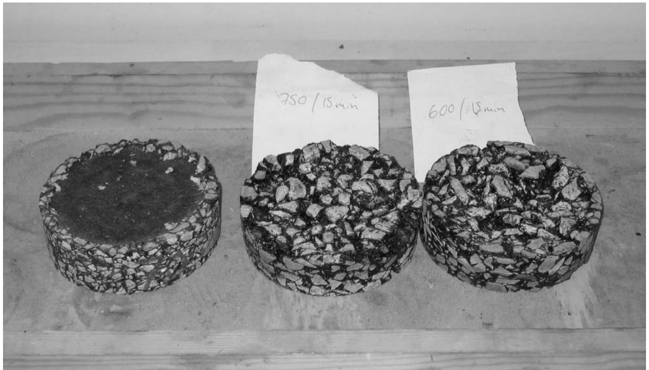
Figure 50: On the left: SMA 5 sample with rubberised bitumen. Bitumen has formed a sheltering cover on the top of the sample. In the middle: open graded asphalt (OA11) after the modified Prall-test (750 rpm/15 minutes). Still the edges of the sample broke. On the right: open graded asphalt (OA11) after the modified Prall-test (600 rpm/15 minutes). Sample has stayed whole but did not wear much. After this the testing time was added to 30 min.
