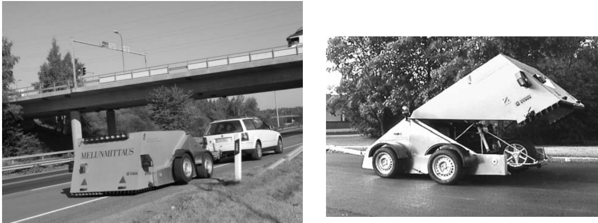
Figure 18: NOTRA®-trailer on the road and the setting of measuring tyre. [Sainio, P. (2002)]
