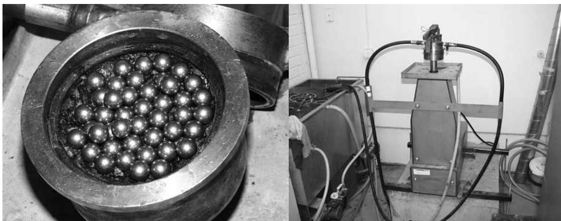
Figure 19: Prall-device. Core samples shall be tested for 15 min with 40 steel balls. Sample shall be rinsed with water during the test.
