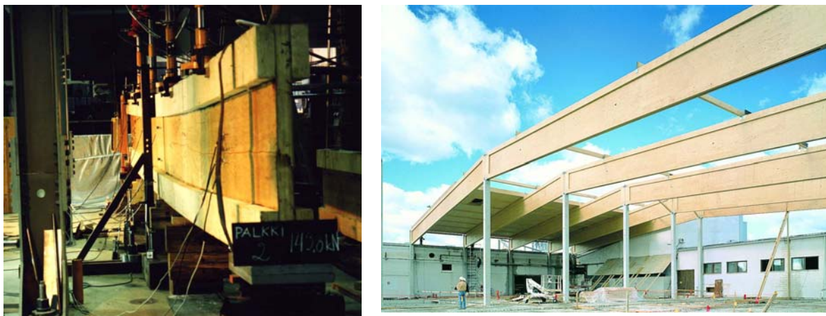
Figure 66. On the left: Maxi-I beam in bending test at HUT/TRT. The beam height was 900 mm, the span was 10.8 m and the achieved breaking load was 143.8 kN. On the right: Enlargement of Kerto-LVL unit in 1997. The span of the main beams is 26 m and spacing 6 m (source:Finnforest).
