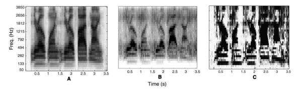
Fig. 2. (A) Rate map for the male utterance "zero one zero five nine" without added noise. (B) Rate map for the same utterance in the presence of noise with an SNR of 5 dB. (C) Soft SNR mask (black pixels are reliable, white pixels are unreliable).
