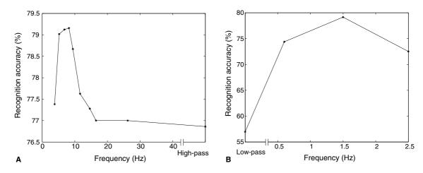
Fig. 5. Tuning the modulation bandpass filter. The graphs show recognition accuracies averaged over 300 test utterances, each convolved with three room impulse responses. (A) The 3 dB highpass cutoff frequency was fixed at 1.5 Hz and the lowpass cutoff was varied. The last data point in the graph represents a plain highpass filter. (B) The lowpass cutoff frequency was fixed at 8.2 Hz and the highpass cutoff was varied. The first data point represents a plain lowpass filter.
