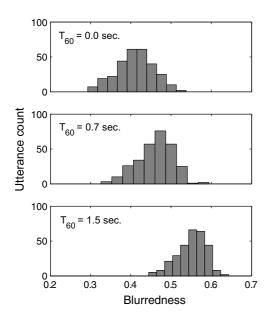
Fig. 6. Distributions of blurredness B for three reverberation conditions, computed from a test set of 300 utterances.
