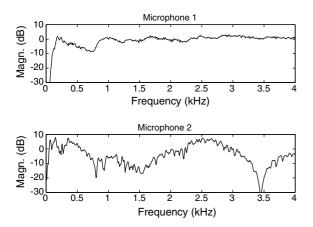
Fig. 8. Frequency responses of the two microphones used in the second experiment.
