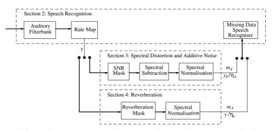
Fig. 1. Schematic diagram of the system. In the processing pathway described in Section 3, a mask  $m_s$  is derived from local SNR estimates, and this is passed to the recogniser together with a 'cleaned' rate map  $y_s$ , which is normalised by a factor  $\eta_s$ . In the pathway described in Section 4, a reverberation mask  $m_r$  is estimated and this is passed to the recogniser together with the rate map y, normalised by a factor  $\eta_r$ .
