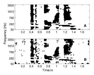
Fig. 3. Selection of time-frequency regions for spectral normalisation, for the male utterance "seven two one nine" when (A) clean and (B) mixed with subway noise at a SNR of 5 dB. Black areas correspond to the regions selected for scaling according to the *L*-largest rule.
