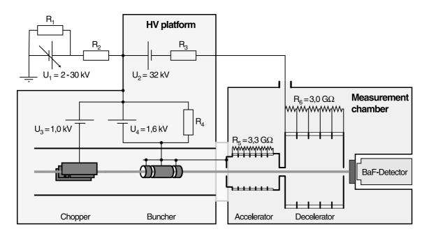
Figure 1: High voltage diagram of the lifetime beam.
