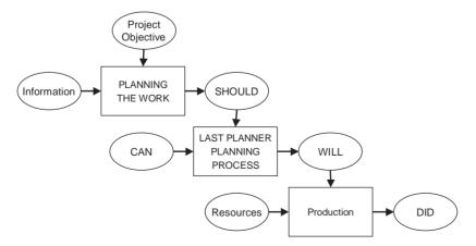
Fig. 1. The Last Planner System (Ballard, 2000).
