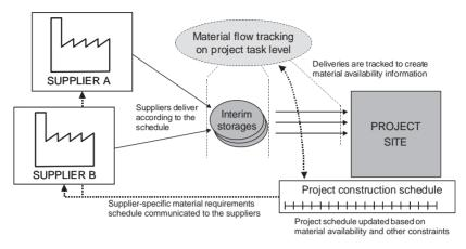
Fig. 6. An illustration of the proposed material delivery system.
