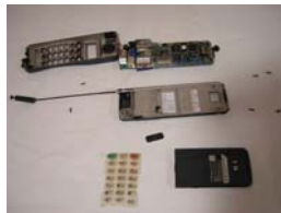
Figure 5: Product dissection example (cellular phone, OKI, 1998)
