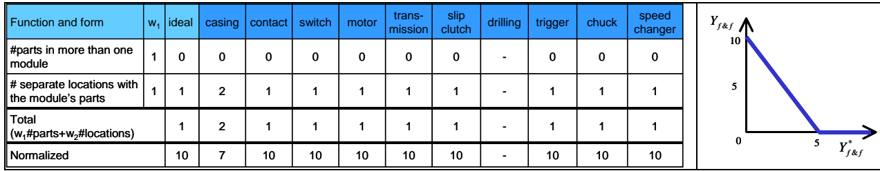
Figure 2 Evaluation of Function-Form alignment for the drill platform.
