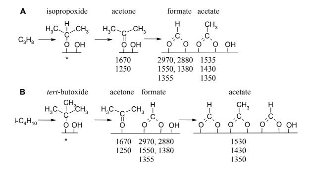
**Figure 6.** Formation of oxygen-containing carbon species during reduction of chromia/alumina with (A) propane and (B) isobutane [III, IV, 50]. Approximate structures based on [63]. Wavenumber values are in units of  $cm^{-1}$ . The scheme does not reflect the real stoichiometries of the reactions. \*The species was not detected but was assumed to form in accordance with [63].
