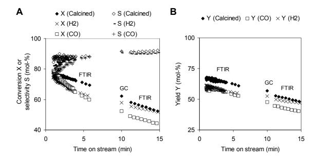
**Figure 7.** (A) The conversion of isobutane (X) and selectivity to isobutene (S), and (B) the yield of isobutene (Y) for the 13.5Cr/Al catalyst after calcination and after H<sub>2</sub> or CO prereduction at 580 °C, 1.03 bar, WHSV=5 h<sup>-1</sup> and nitrogen dilution 1 mol/9 mol. [IV]
