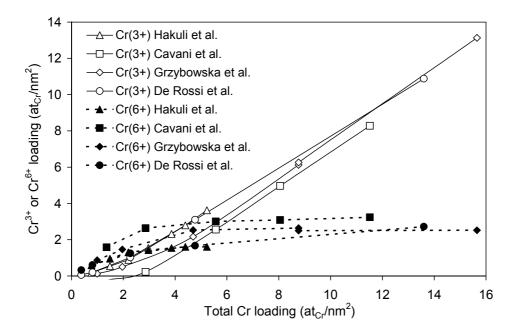
**Figure 1.** Correlation between the total chromium loading and the  $Cr^{3+}$  and  $Cr^{6+}$  loadings for different chromia/alumina catalysts as determined by Hakuli et al. [25], Cavani et al. [26], Grzybowska et al. [27] and De Rossi et al. [28].
