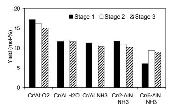
**Figure 2.** Yield of isobutene at 10 min on isobutane stream with the Cr/Al-*Y* and Cr/n·AlN-NH<sub>3</sub> catalysts as measured by GC at 580 °C, 1.03 bar, WHSV=15 h<sup>-1</sup> and nitrogen dilution 3 mol/7 mol. [I]
