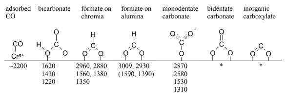
**Figure 5.** Carbon-containing species formed on chromia/alumina during carbon monoxide reduction [II, IV]. Approximate structures based on [59, 60]. Wavenumber values are in units of  $\text{cm}^{-1}$ . \*Species possibly present. *n*=3 (and possibly 2).
