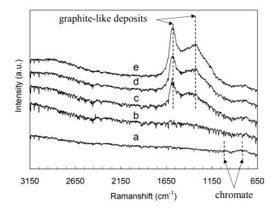
**Figure 9.** Raman spectra measured for the calcined 13.5Cr/Al catalyst at 580 °C (a) after calcination, and during the propane dehydrogenation measurement after (c) 10, (d) 20, (e) 30 and (f) 40 min on propane stream. Spectra measured after helium flush. [III]
