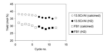
**Figure 11.** Yield of isobutene in 12 consecutive isobutane dehydrogenation stages for the 13.5Cr/Al and FB1 catalysts after calcination or H<sub>2</sub> prereduction at 10 min on isobutane stream at 580 °C, 1.03 bar, WHSV 15  $h^{-1}$  and nitrogen dilution 1 mol/1 mol. [V]
