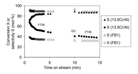
**Figure 10.** Conversion of isobutane (X) and selectivity to isobutene (S) for the 13.5Cr/Al and FB1 catalysts in dehydrogenation of isobutane at 580 °C, 1.03 bar, WHSV 15  $h^{-1}$  and nitrogen dilution 1 mol/1 mol. [V]
