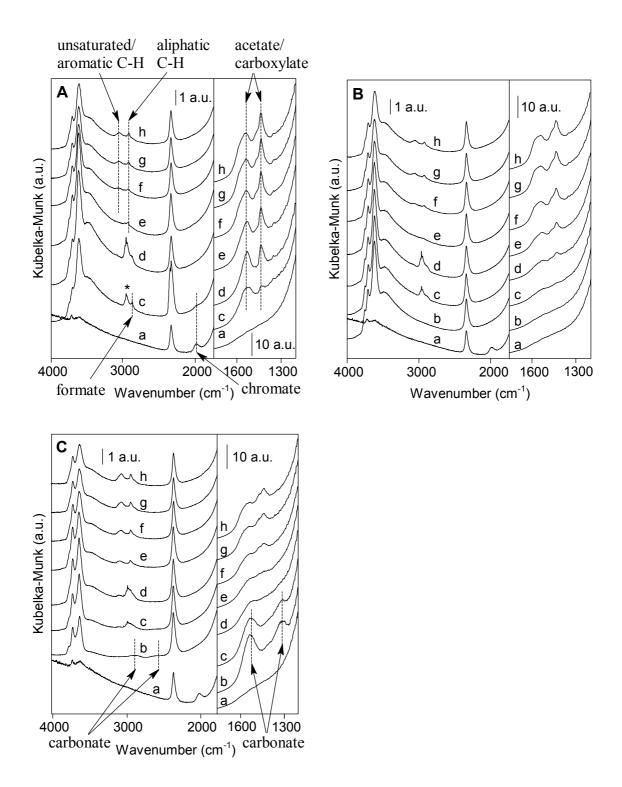
**Figure 8.** DRIFT spectra measured for (A) calcined, (B)  $H_2$ -prereduced and (C) CO-prereduced 13.5Cr/Al catalyst at 580 °C (a) after calcination, (b) after  $H_2$  or CO prereduction, and during the isobutane dehydrogenation measurement after (c) 10 s, (d) 1 min 10 s, (e) 3, (f) 6, (g) 10 and (h) 15 min on isobutane stream. Spectra (c) and (d) measured under isobutane flow and spectra (e)–(h) after nitrogen flush. \*Gaseous isobutane. [IV]
