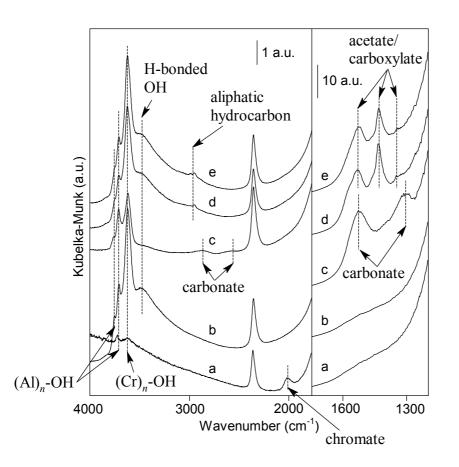
**Figure 3.** DRIFT spectra measured for the 13.5Cr/Al catalyst after (a) calcination, and reduction by (b)  $H_2$ , (c) CO, (d) propane and (e) isobutane at 580 °C. Spectra were measured under inert gas after a 15 min reduction (b and c) or after 3 min on alkane stream (d and e).
