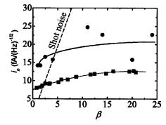
FIG. 2. Experimental ( $\bullet$ ) and simulated ( $\blacksquare$ ) output current noise spectral density as a function of the current gain for base current  $I_B$ =60 pA. Fitted lines are to guide the eyes.
