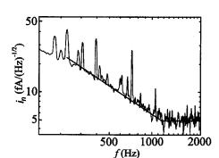
FIG. 4. Input referred current noise spectrum for  $I_B$ =400 pA. The 1/f corner frequency is found at the vertex of the two lines.
