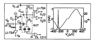
FIG. 1. Left: Measurement setup for the cross correlation and power gain measurements. The BOT circuit is indicated by the dashed box. The BOT and the resistor  $R_{\rm CC}$  are at 34 mK while the rest of the components are at room temperature. Right: I–V characteristic and current gain for  $I_B$ =60 pA. The Coulomb blockade is clearly seen as the environmental resistance  $R_C \gg R_O$ =6.45 kΩ and  $E_J \ll E_C$ .
