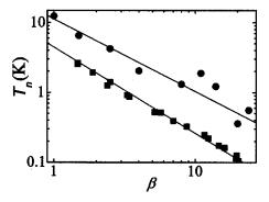
FIG. 3. BOT input referred noise temperature as a function of current gain  $\beta$  from the experiment ( $\bullet$ ) and simulation ( $\blacksquare$ ).
