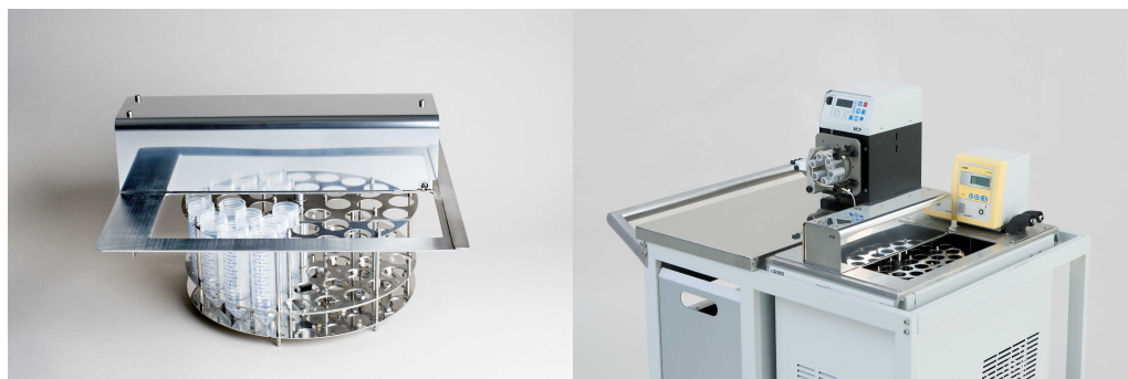
Figure 14. Medical Sampling Unit for automated rapid sampling (© Medical Oy).
