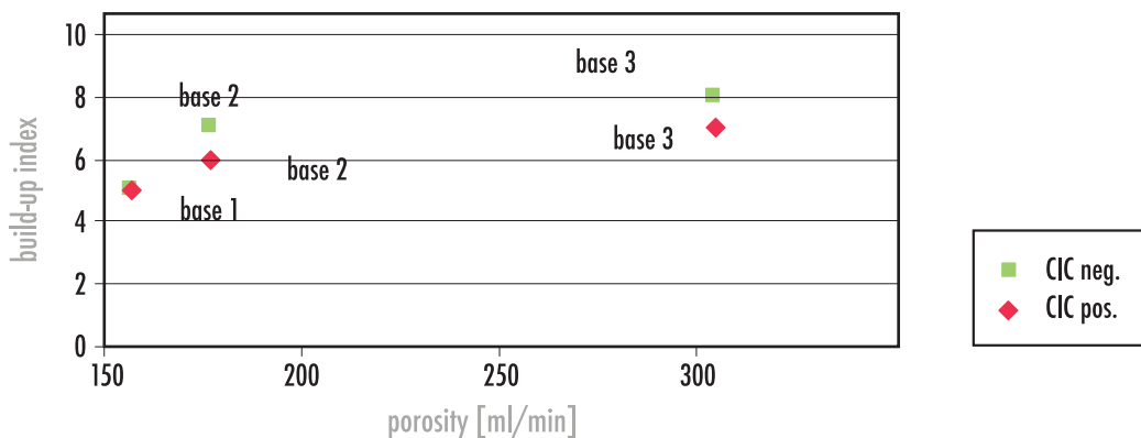
Figure 24. Positive and negative build-up index (higher index=smaller build-up tendency) as function of base paper porosity.
