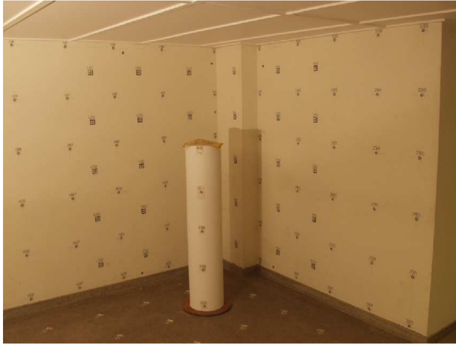
Figure 17. Three-dimensional calibration field used in calibration.
