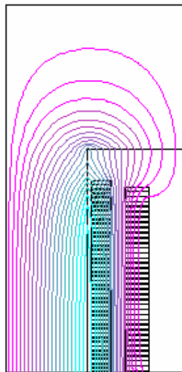
Fig. 4.4 Stray field pattern for windings inside the core
