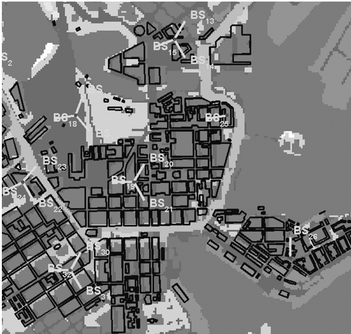
Fig. 3. The pure small macro cell scenario with five three-sector and two one-sector macro cell sites in Helsinki center area. Water areas are shown in blue. Average site distance roughly 910 m. Subset of 32-cell scenario in Reference [26].
