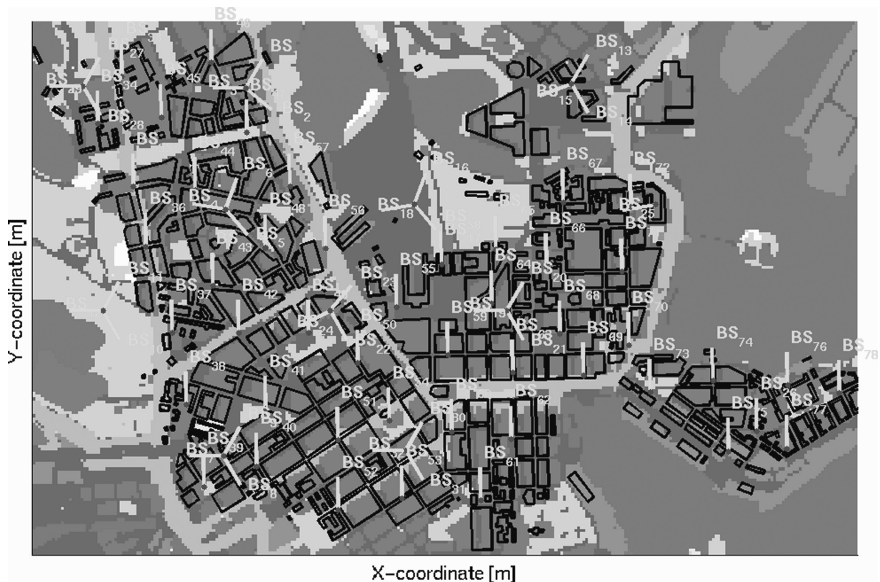
Fig. 4. Mixed micro and micro case with 32 macro cells and 46 micro cells deployed in Helsinki center area.
