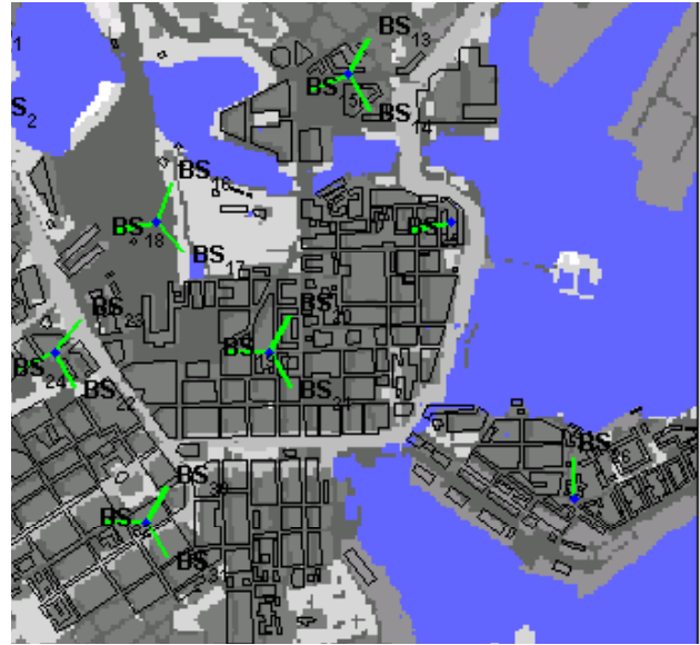
Fig. 1. The case 1 deployment of five three-sector and two one-sector macro cell sites in Helsinki center area. Water areas are shown in blue. Average site distance roughly 910 m. Subset of 32-cell scenario in [5] p. 119.
