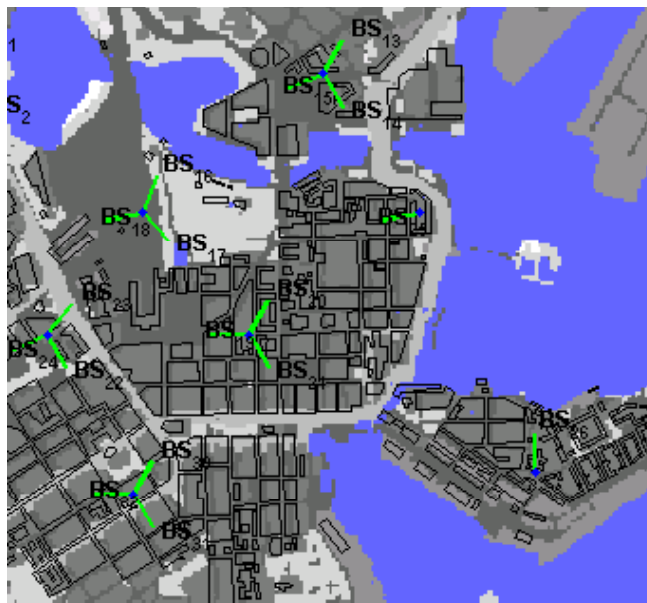
Fig. 1. Deployment of five three-cell and two one-cell macro cell sites in Helsinki center area. Water areas are shown in blue. Average site distance roughly 910 m. Subset of 32-cell scenario in [3] p. 119.
