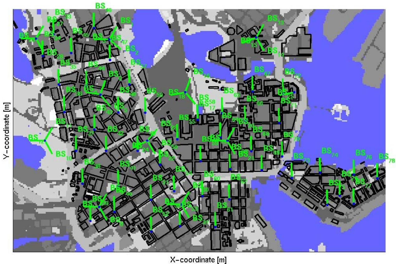
Fig. 4: Deployment of 32 macro cells and 46 micro cells in Helsinki center area.
