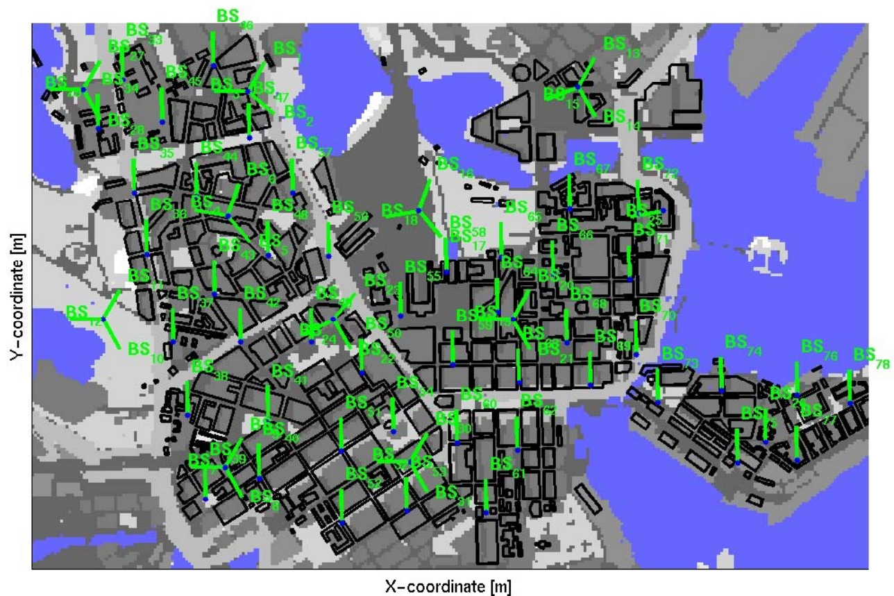
Fig. 3. Deployment of 32 macro cells and 46 micro cells in Helsinki center area. Water areas are shown in blue.
