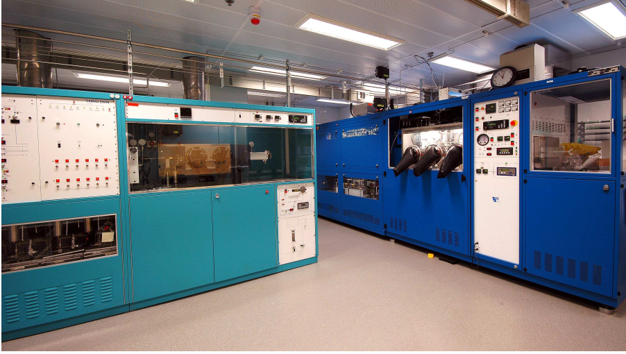
Figure 2.3. MOVPE systems supplied by Thomas Swan Scientific Equipment installed in Optoelectronics laboratory, Micronova.
