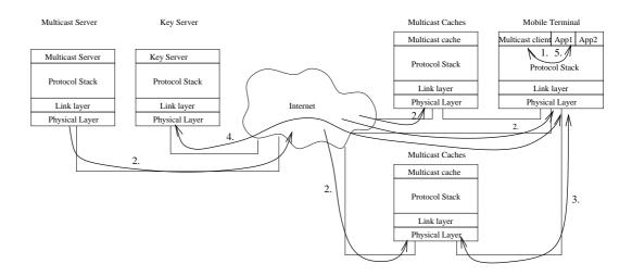
Figure 5: High-level view of the delivery architecture.
