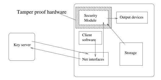
Figure 17: Security module in hardware
