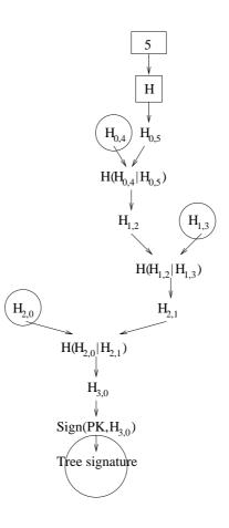
Figure 9: Example of receiver source authenticating packet with sequence number 5.
