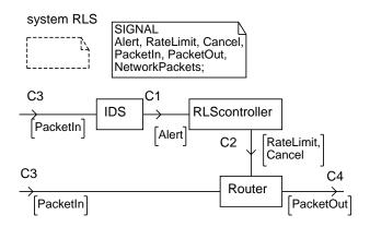
Figure 1. The SDL system diagram for a Rate-Limiting System (RLS) consisting of an IDS, an RLS controller, and a router with QoS-support.
