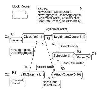
Figure 2. The SDL block diagram for a router in an RLS.
