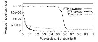
Figure 5. The average TCP throughput in the simulator. A flooding DDoS attack was in the background.
