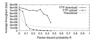
Figure 6. The average TCP throughput measured from the test system. No background traffic was present.
