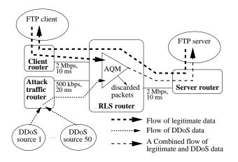
Figure 3. The topology of the simulated network. The dotted lines indicate the flow of data. The AQM in the RLS router discards a specific fraction of packets being sent to the FTP server. No packets are discarded by RLS in the reverse direction.
