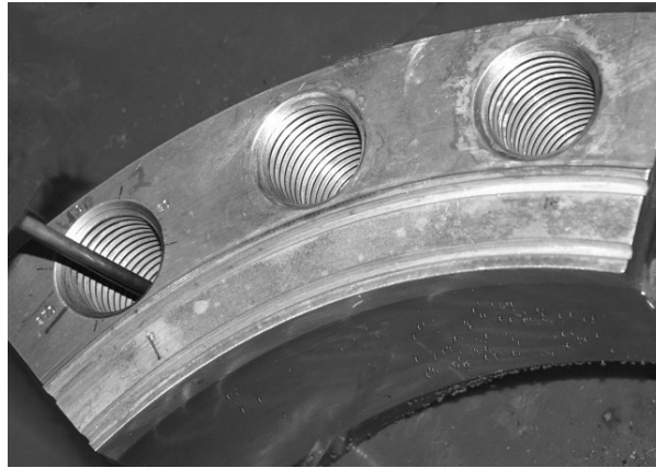
Figure 11. Production of cracks inside of an austenitic stainless steel collector head threaded screw hole.
