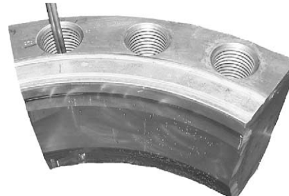
Fig. 18. Production of artificial thermal fatigue cracks inside of austenitic stainless steel collector head threaded screw hole.
