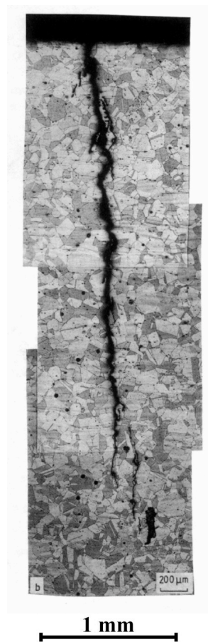
Figure 3 A cross-sectional view of a service-induced thermal fatigue crack in austenitic stainless steel pipe of water clean-up system of a BWR (Hänninen et al., 1981).
