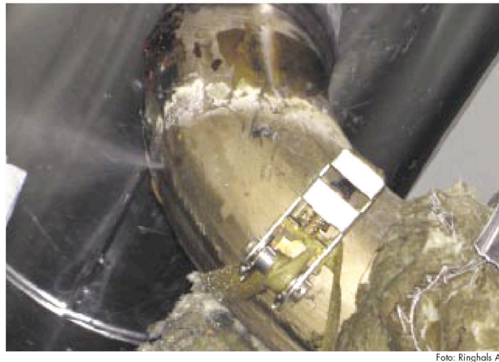
Figure 1 Service-induced thermal fatigue crack causing leakage in a BWR reactor pipe elbow of the reactor water clean-up system (SKI, 2005).
