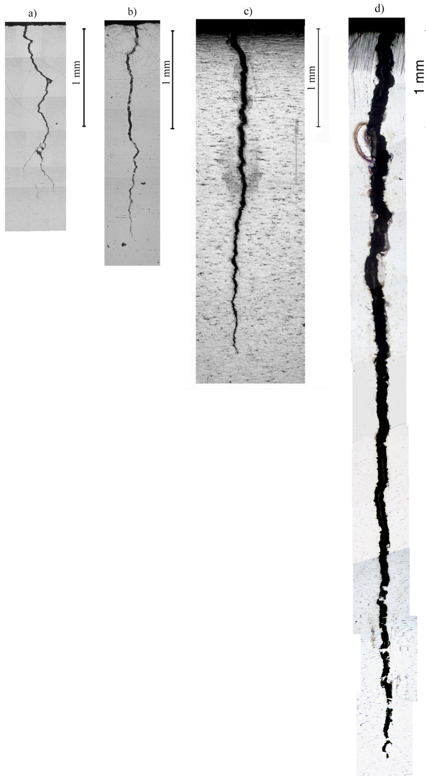
Figure 41 Four different flaws in AISI 304 austenitic stainless steel samples produced by the developed method. Flaws after approximately a) 30 000, b) 2770, c) 6500 and d) 167 000 thermal fatigue cycles.
