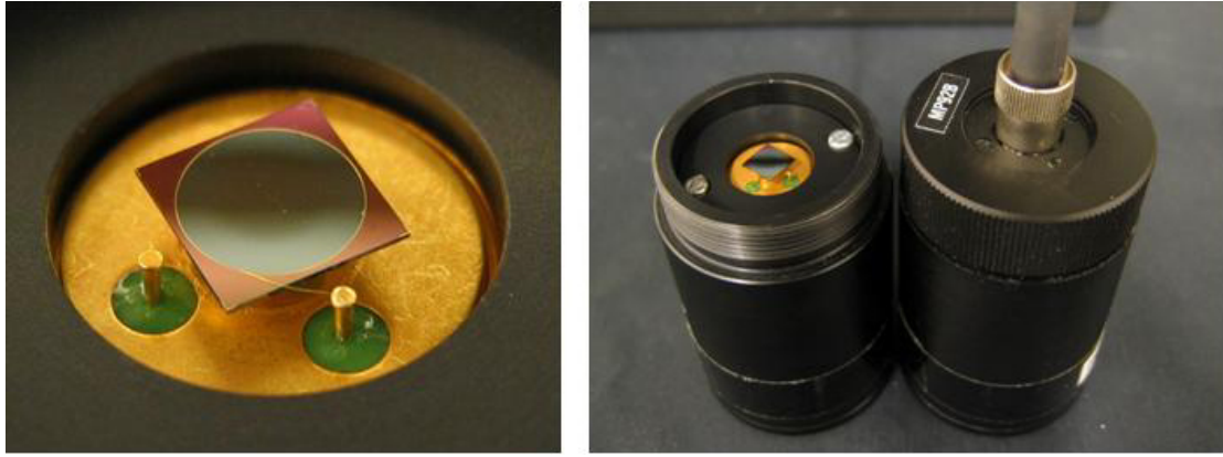
Figure 10. On the left: close-up of the InGaAs photodiode GAP5007 (Germanium Power Devices Inc.). On the right: assembled detectors with plain photodiodes with and without the fiber adapter.
