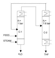
Fig. 3. Separation of THF/water mixture in two-column system.
