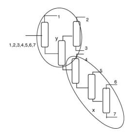
Fig. 4. The synthesised separation sequence (Solution 1).
