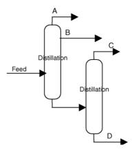
Fig. 7. The train with a combined operation.
