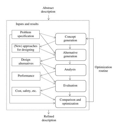
Figure 2.1 The steps of process synthesis (modified from Biegler et al. 1997)
