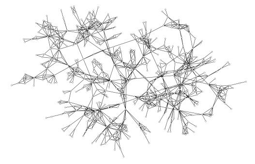
Fig. 2. A visualization of a small network with N = 500 indicates strong community structure with communities of various sizes clearly visible. The number of initial contacts is distributed as  $p(n_{init}=1) = 0.95$ ,  $p(n_{init}=2) = 0.05$ , and the number of secondary contacts from each initial contact  $n_{2nd} \sim U[0,3]$  (uniformly distributed between 0 and 3). The network was grown from a chain of 30 vertices. Visualization was done using Himmeli [36].
