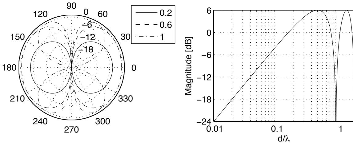
Figure 2.5: Logarithmic magnitude responses of an ideal gradient microphone according to Eq. (2.6). Left: Polar plots as a function of  $\theta$  for  $d/\lambda = 0.2, 0.6, 1$ . Right: Magnitude response for  $\theta = 0$  as a function of  $d/\lambda$ .
