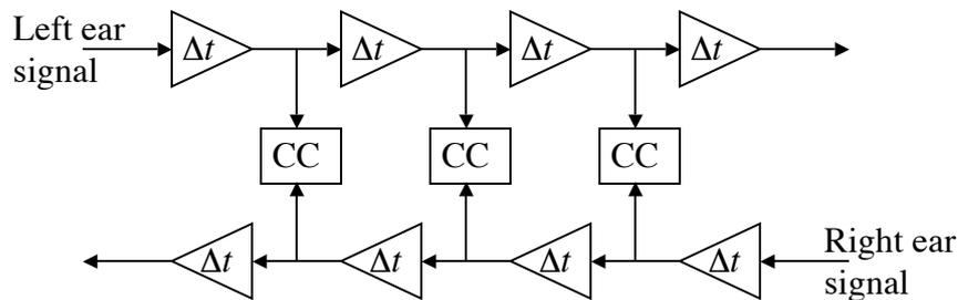
Figure 3.8: Illustration of a Jeffress (1948) coincidence structure for ITD extraction. The  $\Delta\tau$  blocks are delays and the CC blocks depict coincidence detectors. In a cross-correlation model, the coincidence detectors would consist of multiplication and time integration.
