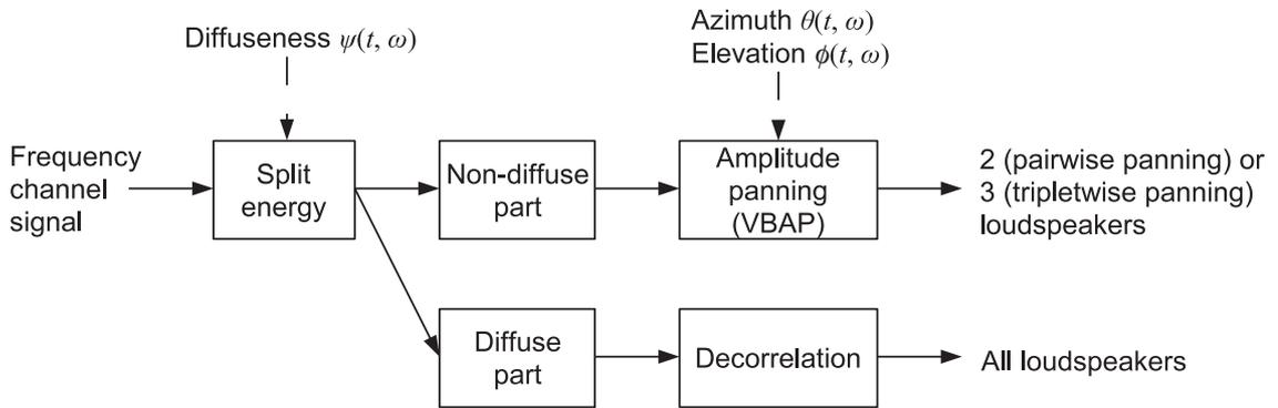
Figure 5.3: Directional synthesis based on an omnidirectional room response: processing of a single frequency channel.
