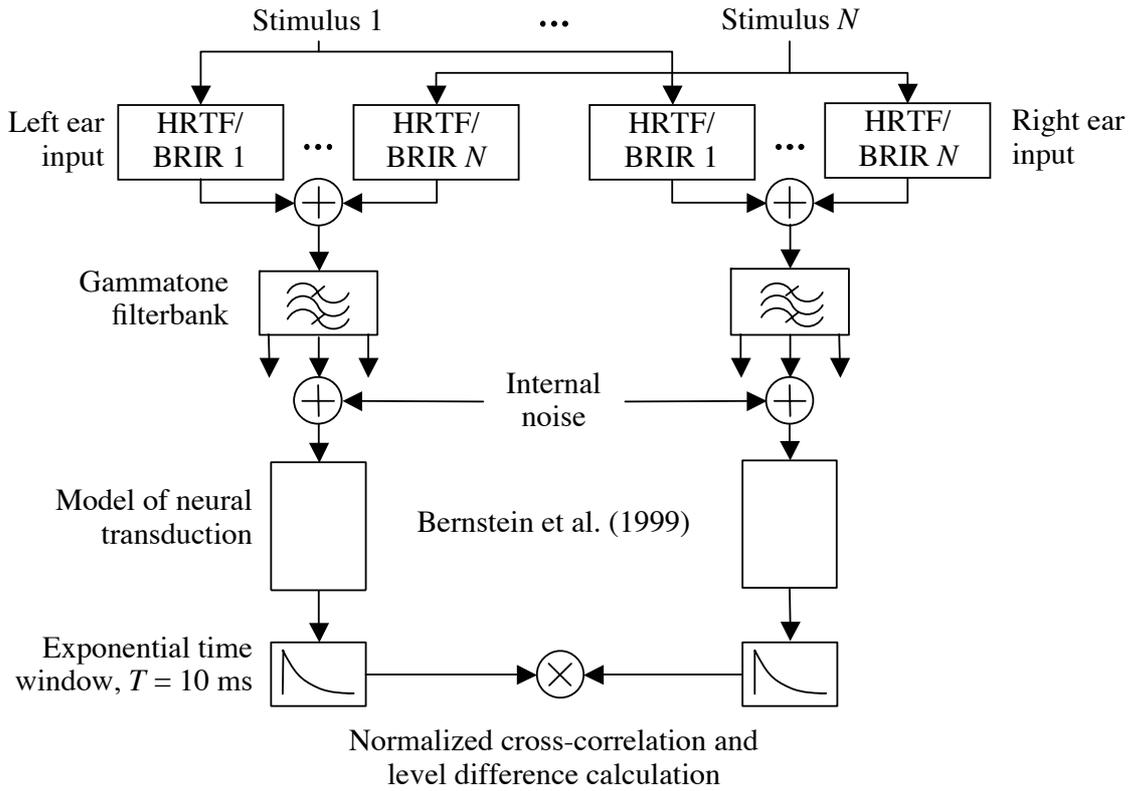
Figure 4.1: Structure of the peripheral part and binaural processor of the cue selection model. For an illustration of the neural transduction part, see Figure 3.7.
