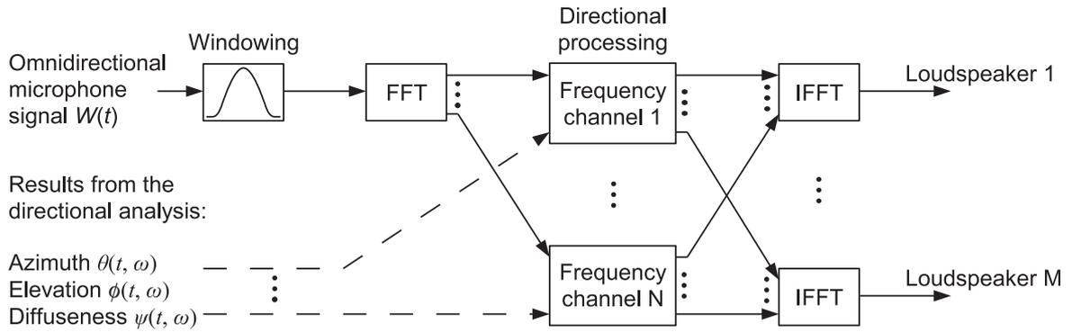
Figure 5.2: Directional synthesis based on an omnidirectional room response: time-frequency processing.
