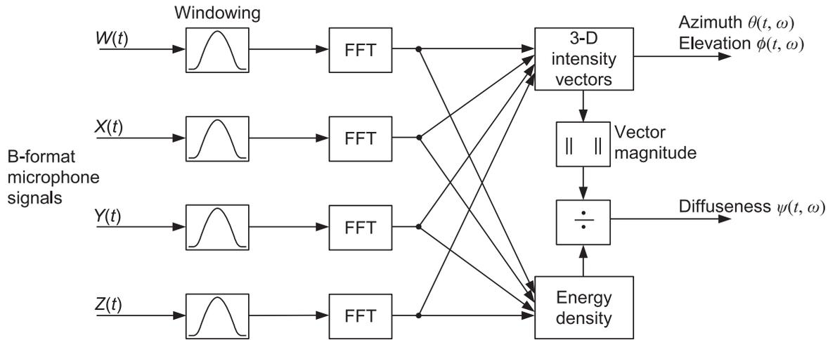
Figure 5.1: Directional energetic analysis of a B-format room response.
