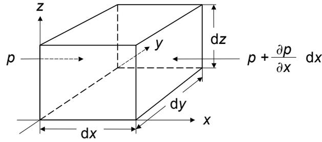
Figure 2.8: A rectangular fluid element with illustration of the forces acting on the  $x$ -axis (after Cremer and Müller, 1982b, p. 3).
