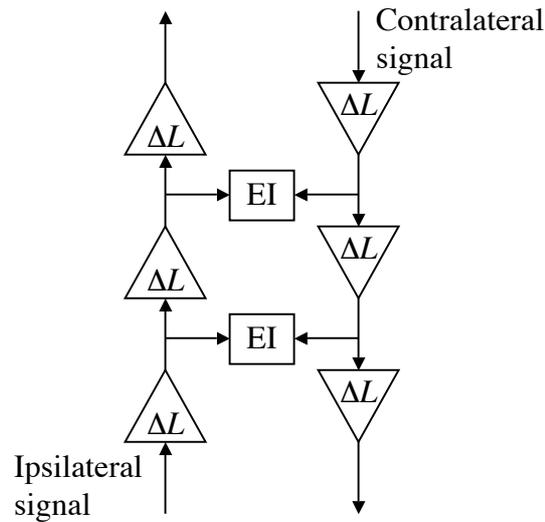
Figure 3.9: Functional view of the ILD extraction model of Reed and Blum (1990) as implemented by Breebaart *et al.* (2001a). The  $\Delta L$  blocks are attenuators and the EI blocks perform subtraction of the contralateral signal from the ipsilateral signal followed by half-wave rectification.
