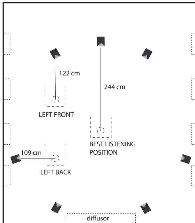
Figure 5.14: The loudspeaker configuration and listening positions in the listening room.
