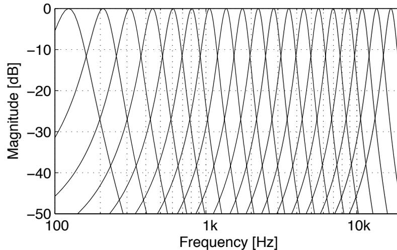
Figure 3.6: Frequency responses of a gammatone filterbank (Slaney, 1998) with a spacing of two ERBs between center frequencies.
