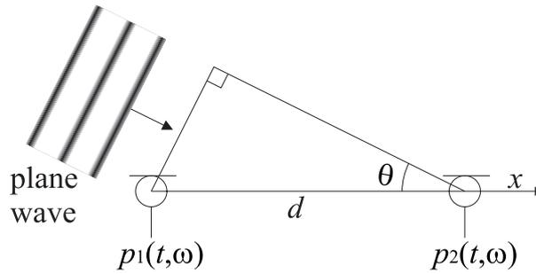
Figure 2.4: Plane wave arriving from angle  $\theta$  to a microphone pair placed on the  $x$ -axis with a distance  $d$  between the microphones.
