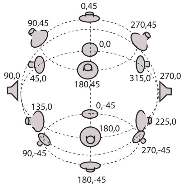
Figure 5.10: The 3-D loudspeaker system employed in the anechoic listening tests. The pairs of numbers describe the azimuth and elevation angles of each loudspeaker, respectively.
