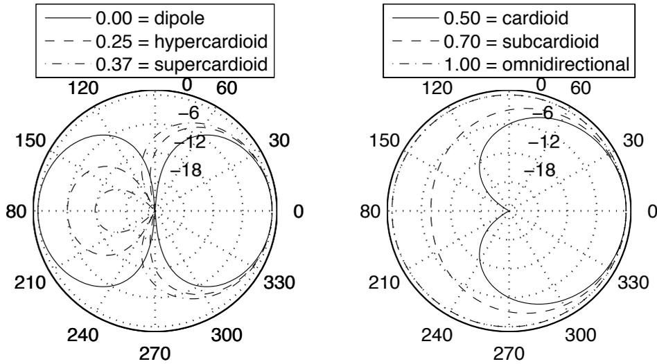
Figure 2.6: Polar plots of the logarithmic magnitude responses of first-order gradient directivity patterns according to Eq. (2.10) with some typical values of  $\beta$ .
