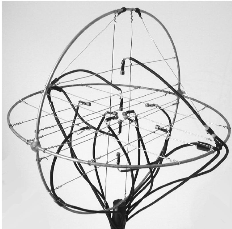
Figure 2.7: TKK 3-D microphone array
