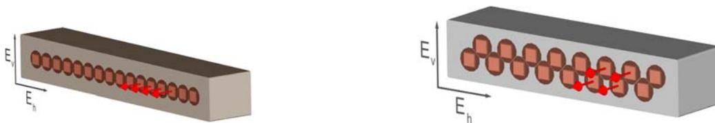
Fig 2. Tx antenna array. The antenna elements used in this work are indicated by arrows. a) Linear array. b) Zigzag array.
