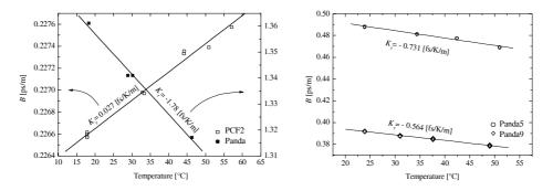
Fig. 4. *B* as a function of temperature @ 1550 nm (averaged over at least 10 nm intervals). Arrows indicate corresponding scales.
