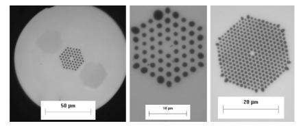
Fig. 1. Cross-sections of the analyzed PCFs. (From left to right) PANDA5 (PANDA7 and PANDA9 have the same cross-section with a different scaling), PCF3, and PCF2.
