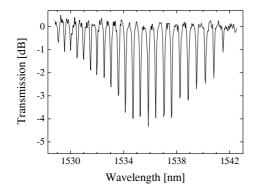
Fig. 10. Normalized absorption spectrum of H<sup>13</sup>CN in a 1 m long PBF1500 recorded using a LED. The resolution of the OSA is 0.1 nm.
