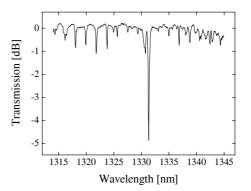
Fig. 11. Normalized absorption spectrum of  $CH_4$  in a 10 m long PBF1300 recorded using a LED. The resolution of the OSA is 0.1 nm.
