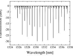
Fig. 6. Normalized absorption spectrum of the Pbranch of  ${}^{12}C_2H_2$  at 10 mbar in a 1 m long PBF1500 measured using a tunable laser (step size 1 pm).
