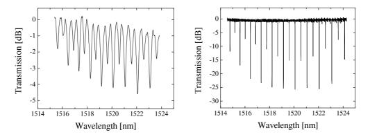
Fig. 8. Normalized absorption spectra of R-branch of  ${}^{12}C_2H_2$  in a 1 m long PBF1500 measured using a LED. The resolution of the OSA is 0.1 nm. The lines appear broader due to the limited resolution of the OSA.
