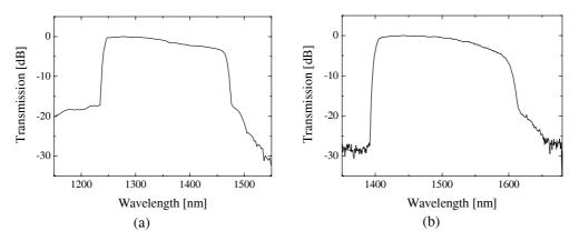
Fig. 2. Spectral transmission of (a) a 2 m long PBF1300 and (b) a 3 m long PBF1500.
