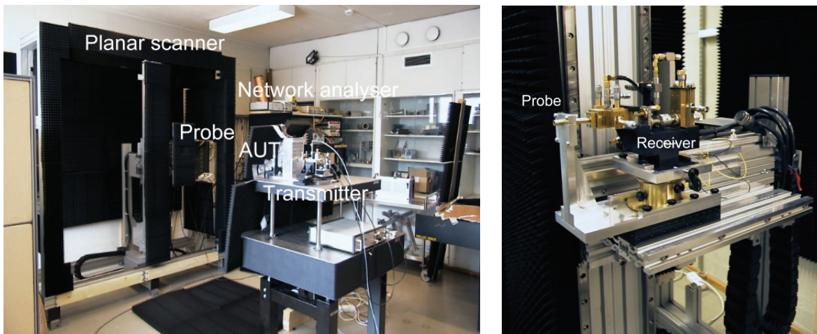
Figure 5.31 DRFS beam measurement set-up and the probe mounting.
