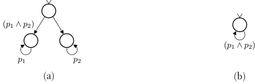
Fig. 5.2: Two automata for the LTL formula  $(Gp_1 \wedge Gp_2)$ . (a) Automaton built for the formula using the basic translation rules; (b) Minimal automaton for the formula
