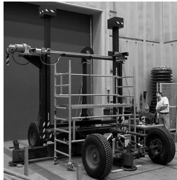
Fig. 9. Plane-Polar quiet-zone scanner mounted on the antenna positioner during instrumentation tests.
