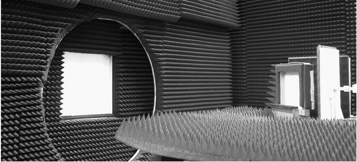
Fig. 3.2. Front view of the phase hologram during quiet zone testing.
