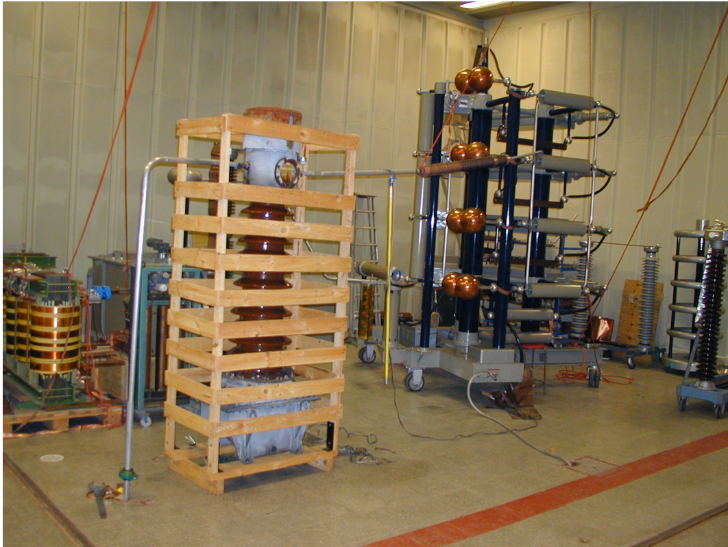
Fig. 52 Impulse measurement of CT4 in the HV laboratory, HUT, Finland.
