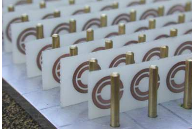
Figure 7: Realization of double-negative material at microwave frequencies [43]
