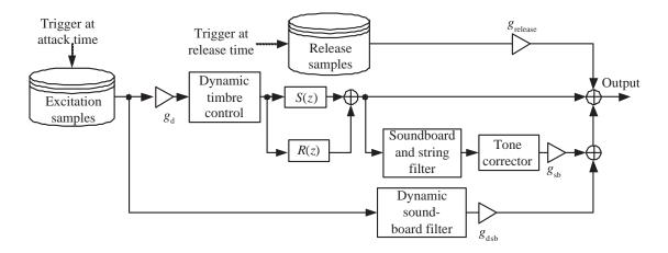
Figure 7: Block diagram of the waveguide synthesis algorithm for the harpsichord with dynamics modeling.
