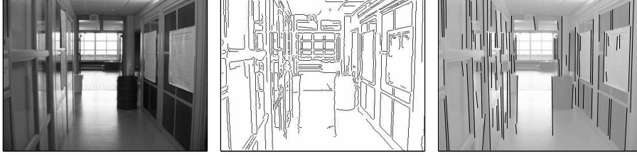
Figure 4.1: Example of the detection of vertical edges. Left to right: Original image, Canny edges and the final edge map.
