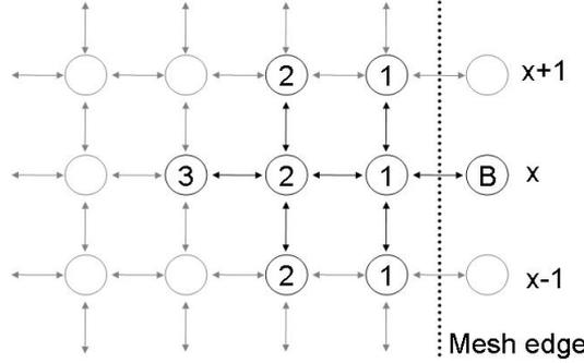
Figure 4.1: In the spatial-filter based absorbing boundary, junctions in a line perpendicular to the boundary and one step to the sides of these junctions are taken into account when updating the boundary junction value.
