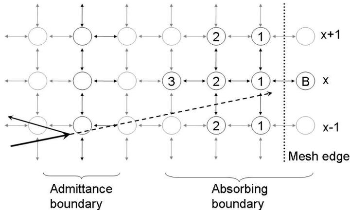
Figure 4.2: The admittance boundary reflects part of the signal, and the rest is absorbed with a spatial-filter based absorbing boundary at the mesh edge.
