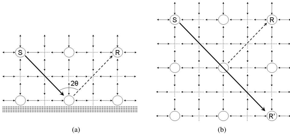
Figure 3.1: The test setup: a) The mesh was initialized at source point S and the output was recorded at receiver points at the same distance from the tested boundary. b) For reference, a perfect reflection was simulated by receiving the signal at mirror locations R' when the mesh was made large enough to prevent any unwanted reflections.
