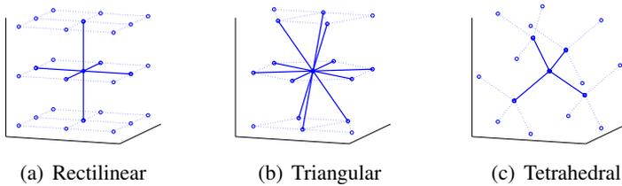
Figure 2.4: Three 3-D mesh topologies.
