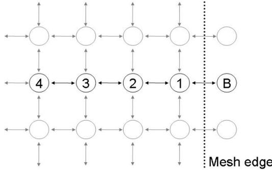
Figure 2.6: Junctions in a line perpendicular to the boundary are used in a Taylor-series absorbing boundary condition.
