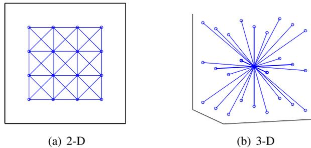
Figure 2.5: In addition to the axial connections, in the interpolated rectilinear topologies the junctions are connected with their diagonal neighbors.
