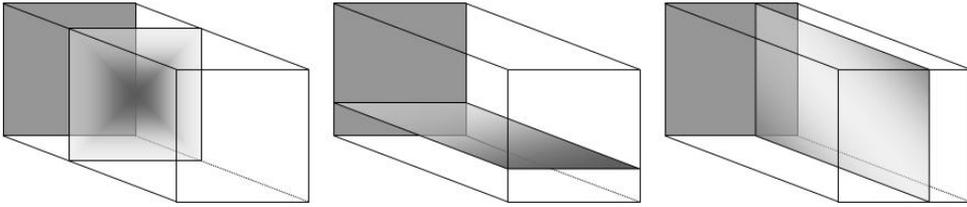
Figure 4.3: Two-dimensional meshes at the cross-sections of a 3-D space for modeling low frequency standing waves.
