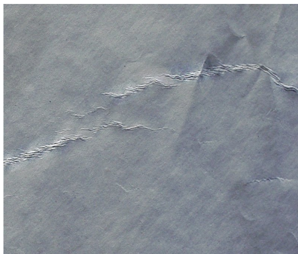
Figure 31: Crepe wrinkles in paper web (photo courtesy of Metso Paper).
