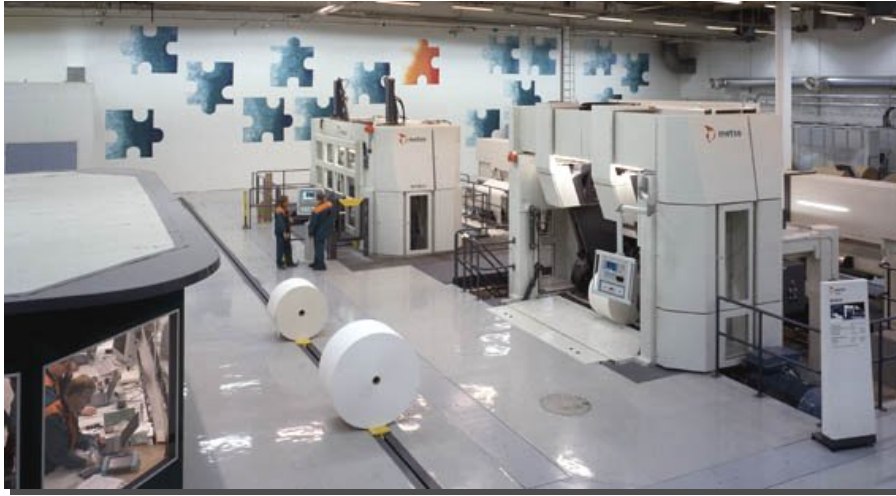
Figure 33: The Winding Technology Center. The multi-station winder in front and two-drum winder used in tests in back (photo courtesy of Metso Paper).
