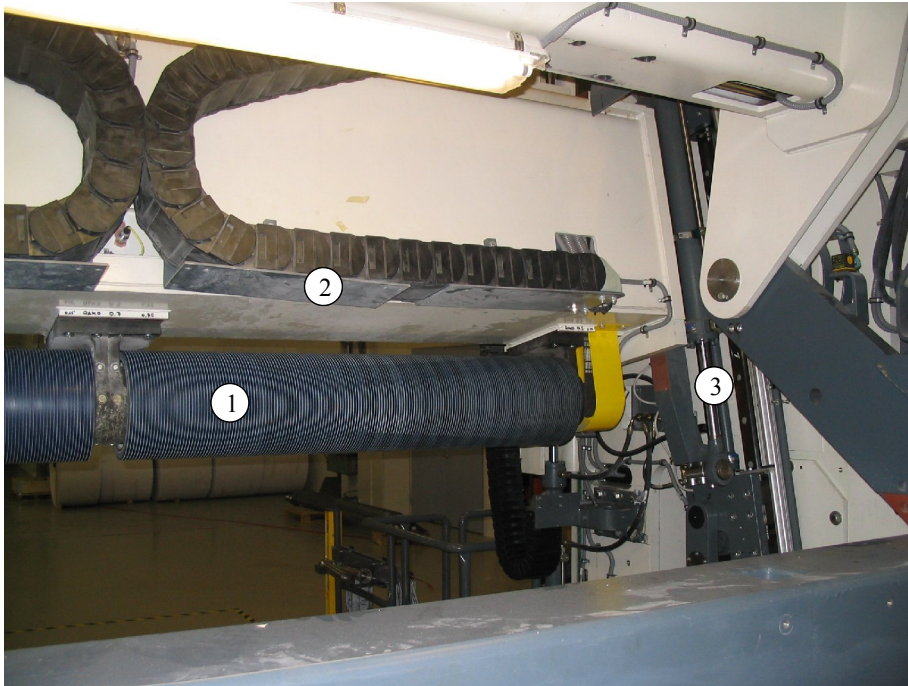
Figure 37: Main parts of the rider roll that presses paper rolls during winding (1=rider roll, 2=rider roll beam and 3=hydraulic cylinder).
