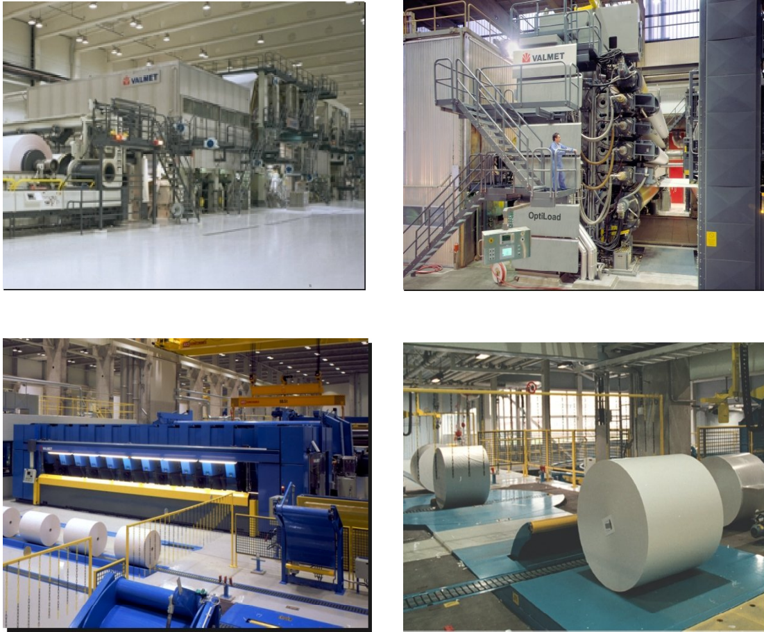
Figure 2: Coater and reel (up-left), multi-nip calender (up-right), paper winder (down-left) and roll handling (down-right). Photos courtesy of Metso Paper.
